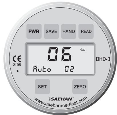
Setting Auto Mode 6 tests (3 per hand) at 2 second intervals
